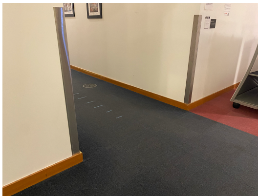
Figure 9: An outside turn scenario where the close proximity of the far wall provides a false positive for the inside turn logic.
