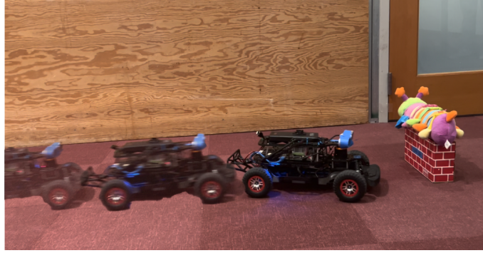
Figure 14: A static obstacle safety test using the stationary brick.
