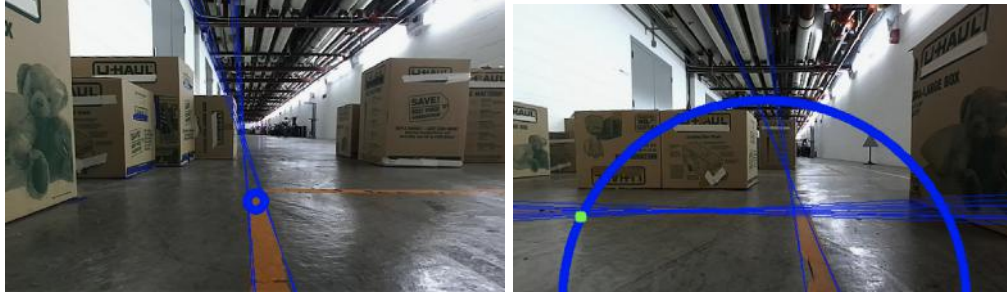
(a) Straight-away case for city driving hough implementation (b) Turning case for city driving hough implementation
