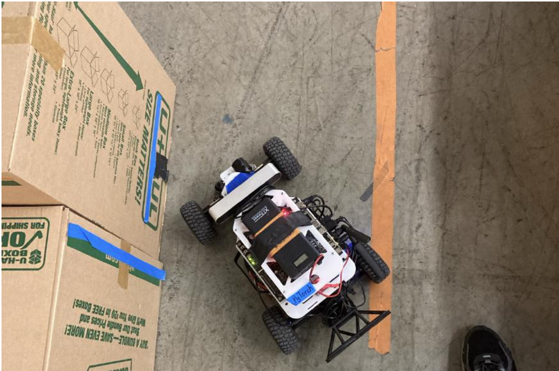
Figure 11: When our color bounds are too loose, our car often ends up mistakenly detecting the bottom of the boxes as the line and skewing the pursuit point in the direction of the boxes. As seen above, the color of the box closely resembles the color of the orange line. It is almost certain that the box color will fall in the orange color bounds if the segmentation is done with insufficient care.
